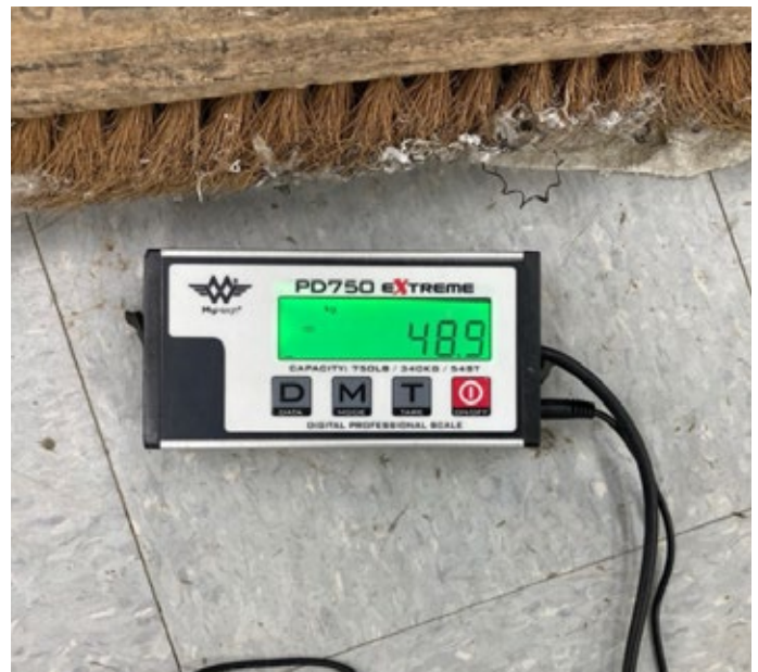
Typical rota-moulded Polyethylene hull weight
