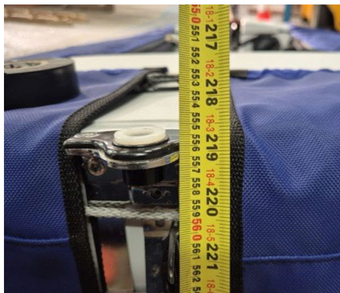
Grey boat mast rake measured as 5560mm
